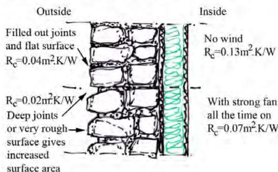
TRANSMISSION RESISTANCE UNDER OPEN ROOF
