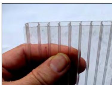
← Polycarbonate fully transparent sheet 6 mm thick
