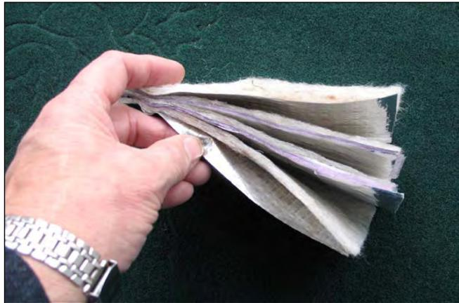
The thermal insulation value of this type of multi-layer insulation is high due to the layers of reflective foil, added with some insulation value of the wool. The wool is resilient and keeps a narrow spacing between the foils in tact, which is necessary to let them reflect the infrared radiation.
