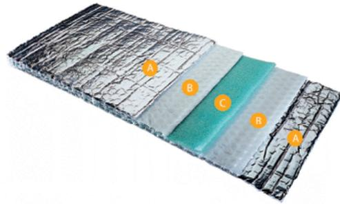
Samples of pre-manufactured thermal insulation products available in the market. Other manufactures reproduce similar products. The 99% pure aluminium reflective foils are more durable and more fire-resistant than the metalized polyester plastic foils. The internal aluminium foils, according to some calculations, do not provide much reflective power or insulation value; but they do substantially increase the cost of the foils.
