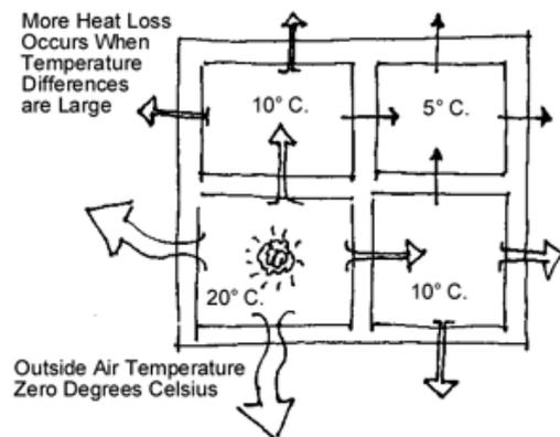
Adjoining rooms and closed unheated roof areas (attic) act as a temperature buffer. The table gives the combined values for the two wall-to-air transfer resistances together. The inside and the outside wall or roof insulation value needs to be added to this value.
