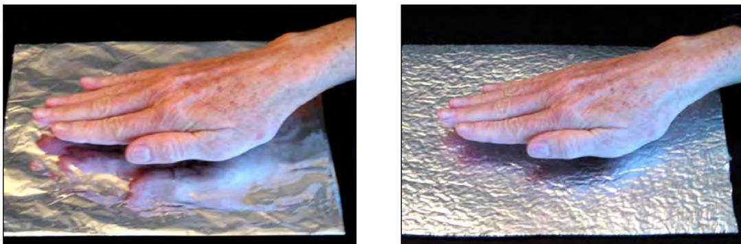
The metallization with aluminium produces a shiny effect and reflects heat radiation (same as infrared radiation). This can be tested by holding your hand low over a reflective foil. The better the heat reflection of the foil, the faster you feel the radiated warmth from your hand bouncing back to you.
