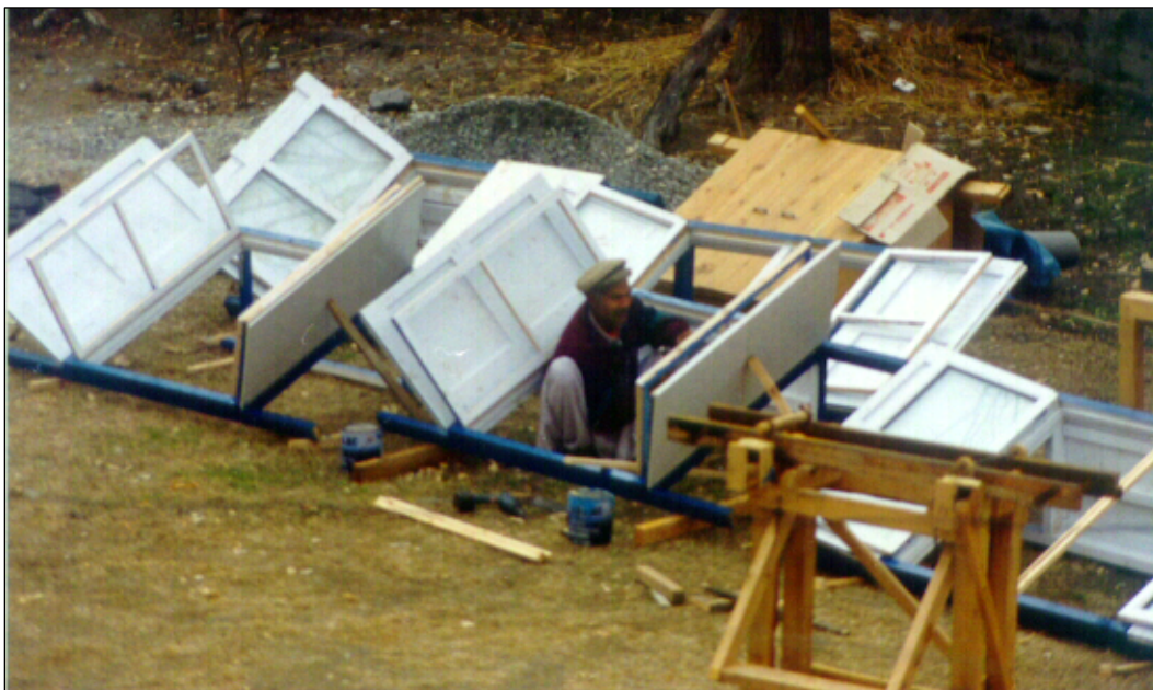
Carpenter Noor making the first series of Roof-Hatch Windows.
