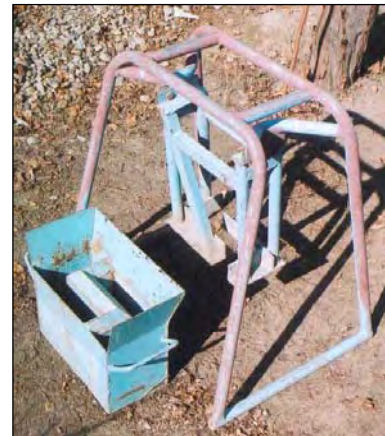
Page from an instruction manual and cement block mould for making the L- and U-corner blocks.
