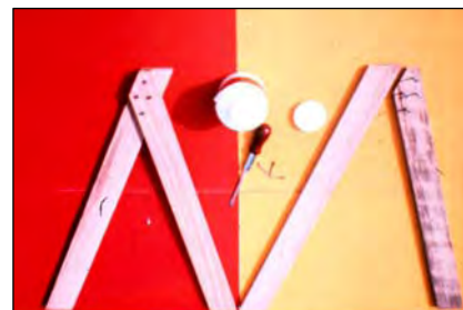
Joints made with PVA glue and screws remain strong, even if timber shrinks.
