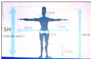
Only the standing height needs to be measured because the size of all other body parts bear a constant relation to it.
