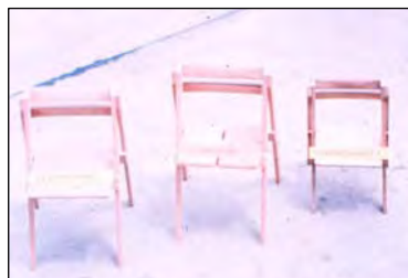
Construction is simple. All timber is the same thickness and width and only two widths are used.
