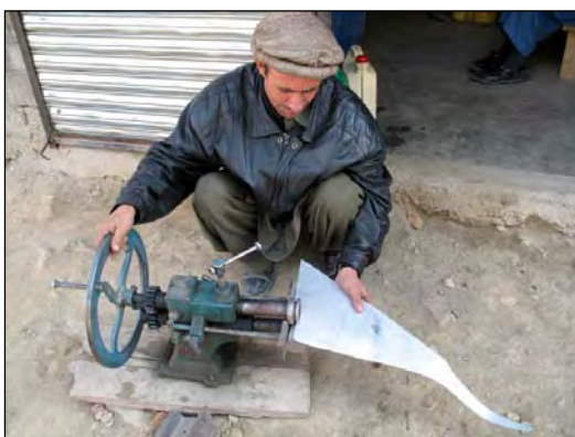
Small hand-operated rolling machine for quickly making sheet steel joints. While machines increase production and can deliver more precise work, their purchase cost needs to be recuperated from increased sales numbers. Large machines can be used by one MSE to supply prefabricated parts to various other MSEs to create a better turnover for the recuperation of the purchase cost.
