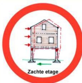
Figures 61. Left: Soft/weak ground floor (shops, terraced houses) with a lot of deformation (high risk).
