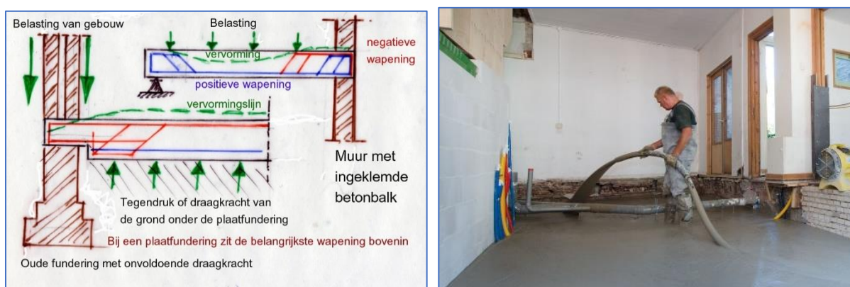
Figures 57. Left. With a concrete beam, a negative moment is created when loaded and clamped in a wall. Here, 'negative' reinforcement is applied (red). With a slab foundation, the load on the building is all around along the edges of the floor, meaning the reverse load of an elevated self-supporting concrete floor. Negative reinforcement must then be placed in the entire top of the slab foundation. Right. Application of foam concrete after foundation repair. https://vandijkmaasland.nl/expertises/schuimbeton/woningbouw/
