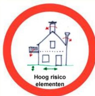
Figures 59. High-risk elements include heavy chimneys on a flexible timber roof structure, balconies wedged into brick walls, and spandrels or free-standing gable ends that sit on buildings and above sidewalks. While falling, they can cause casualties in the public space. Middle and right. Building with high-risk elements: heavy chimney on a weak roof, wedged cantilevered balcony (red), and a building without these high-risk elements (blue). 81
