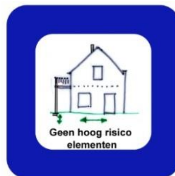
Figures 59. High-risk elements include heavy chimneys on a flexible timber roof structure, balconies wedged into brick walls, and spandrels or free-standing gable ends that sit on buildings and above sidewalks. While falling, they can cause casualties in the public space. Middle and right. Building with high-risk elements: heavy chimney on a weak roof, wedged cantilevered balcony (red), and a building without these high-risk elements (blue). 81
