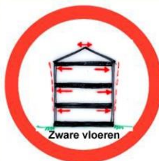
Figures 60. Left. Heavy concrete floors (high risk, red) and Right. light wood floors (low risk, blue).
