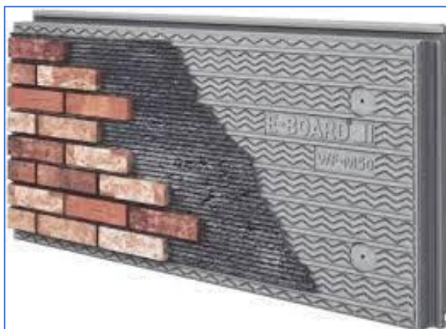
Figure 36. Brick slips can be produced in many (including classic) designs and glued to thermal insulation boards. By adding them with a slightly flexible component adhesive, the load-bearing construction can move slightly without this being visible by cracks in the outer facade. Retrofitted houses will be well insulated and show no more cracks in their facades.
